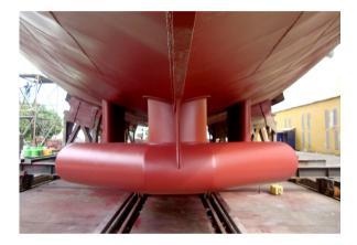
**Figure 2.** Gondola of the arrangement of sensors of the multibeam systems in the lower part of the hull of the vessels ARC Malpelo and ARC Providencia.
