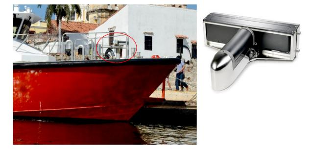
**Figure 4.** MBES on board the ARC Isla Fuerte boat. The arrangement (right) is deployed towards the bow and is submerged in the water when the system operation starts.
